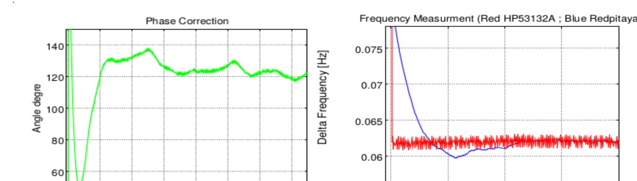
For the sake reconfigurability and ease development, we present here simple tests on medium quality quartz oscillator while data analysis is performed through the embeded CPU unit. Concurrent RAM transfert and calculations benefits from multithreaded techniques
